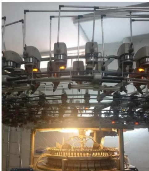
Figure 10: Indicator lights for online measurement
